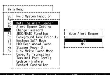
The Mute The Alert Beeper function item is used to control the RAID subsystem Beeper. Select the **Yes** and press **Enter** key in the dialog box to turn the beeper off temporarily. The beeper will still activate on the next event.
