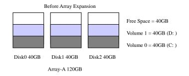
The RAID subsystem controller redistributes the original volume set over the original and newly added disks, using the same fault-tolerance configuration. The unused capacity on the expand raid set can then be used to create an additional volume sets, with a different fault tolerance setting if user need to change.
