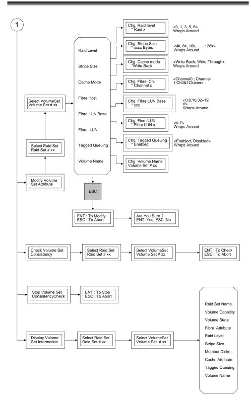
All value can be modifying by the user. Press the **UP/DOWN** to select attribute. Press the **ENT** to modify the default value. Using the **UP/DOWN** to select attribute value and press the **ENT** to accept the selection value. Choose this option to display the properties of the selected Volume Set; you can modify all values except the capacity.
