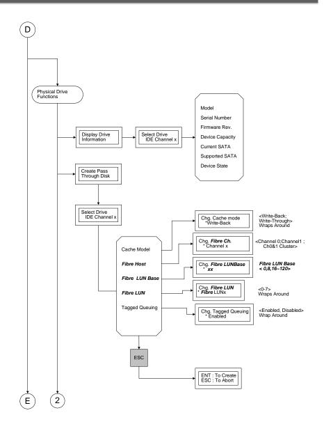
Press **UP/DOWN** to choose the **Display Drive** Information option, then press **ENT** key. This menu will show all physical drive number items. Using **UP/DOWN** to select the Disk that user want to display and press **ENT**, then Press **UP/DOWN** to browse the HDD's information.
